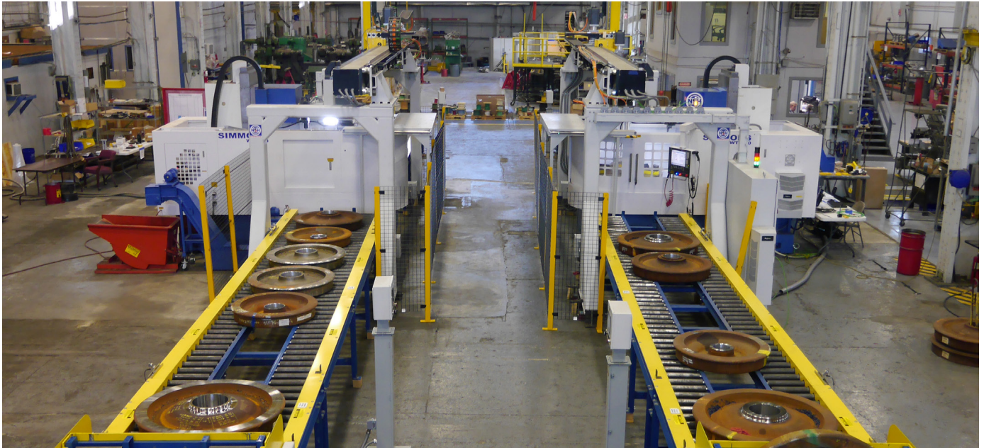
Figure 1: Wheel sets requiring machining are placed onto a conveyor and transported into the machine cell. To accomplish this task, each individual wheel is picked by a vertical lift system from Güdel. The system consists of a ZP-6 overhead gantry with a two-axis robot that has a Simmons specialized gripper to handle the heavy wheels. The system transfers the wheels to the Wheel Turning Center.
